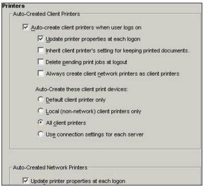
A."Auto-Creating Client Printers when user logs on" is enabled.
