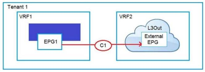
An engineer must have communication between EPG1 in VRF1 and External EPG in VRF2. Which three actions should be taken for the defined subnets in the L3Out External EPG to accomplish this goal? (Choose three.)
