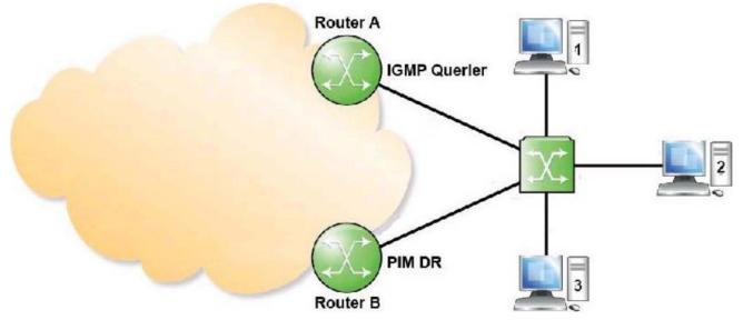
The switch is not igmp-snooping/proxy capable.
