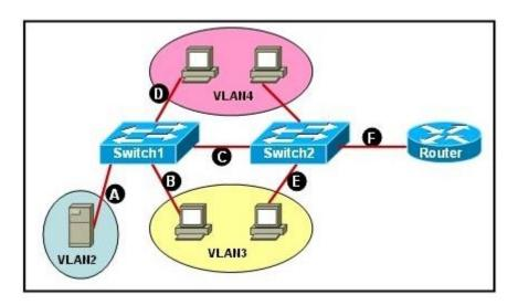
A network associate needs to configure the switches and router in the graphic so that the hosts in VLAN3 and VLAN4 can communicate with the enterprise server in VLAN2.
