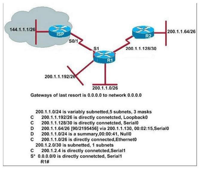
Based on the output of the R1#show ip route command and the information presented in the graphic, which of the following is a potential routing problem?
