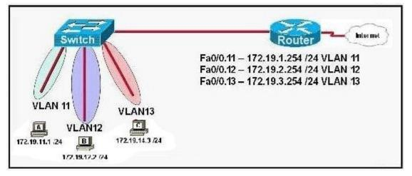
The network shown in the exhibit has just been installed. Host B can access the Internet, but it is unable to ping host C.
