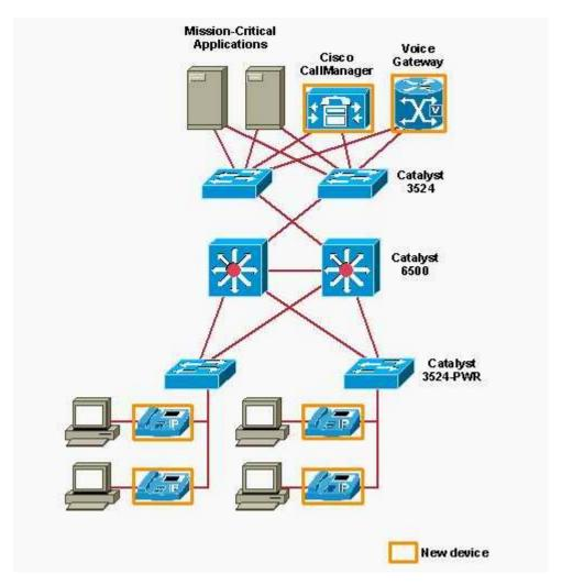
A.The trust boundary should be extended from the 3524-PWR access switches to include the IP phones. B.Ingress rate-limiting should be configured on 3524-PWR access switches to ensure Voice over IP bandwidth guarantees.
