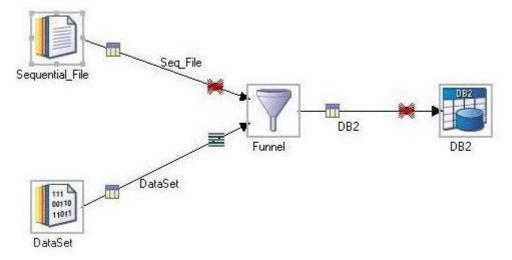
The parallel configuration file contains 4 nodes. How many instances of the Funnel stage run in parallel? A.1
