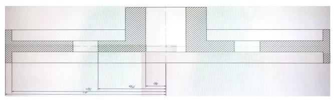
This section view was dimensioned using Baseline Dimensions The dimensions are too close together which impacts the drawing's legibility.
