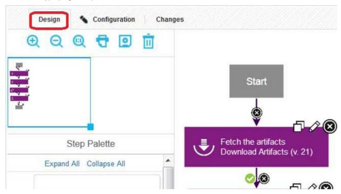
Note: A component process is a series of user-defined steps that operate on a component's artifacts. Each component has at least one process and can have several. Component processes are created with the process editor. The process editor is a visual drag-and-drop editor that enables you to drag process steps onto the design space and configure them as you go. Process steps are selected from a menu of standard steps.
