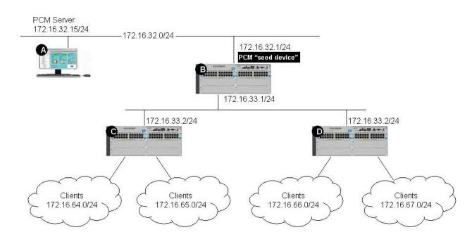
You have installed PCM+ and all of its plug-in applications on the network shown in the exhibit. You have not performed any additional configuration. Which device(s) will be included in the network map when you log in to PCM+ for the first time?
