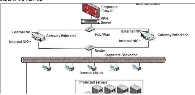
A Symantec Network Access Control administrator is trying to implement two Gateway Enforcers in failover mode. The administrator has implemented the two Enforcers in the network as shown in the exhibit. After starting both Gateway Enforcers, the administrator finds that both Enforcers are in active mode. What is the likely cause of the problem?
